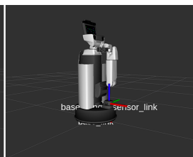
(b) The base_link coordinate system of the HSR. X (red) is forward, Y (green) is left and Z (blue) is up. The base_range_sensor_link (the scanner.link) is in line with the base_link and not rotated.
